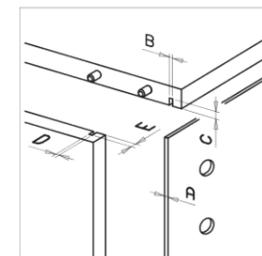
Presence and thickness of the back panel (A), thickness and depth of the milling in the top panel (B, C), thickness and depth of the milling in the side panel (D, E).
